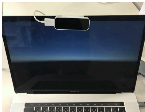
Fig. 5: LEAP Motion Controller device placed on a notebook computer display.
