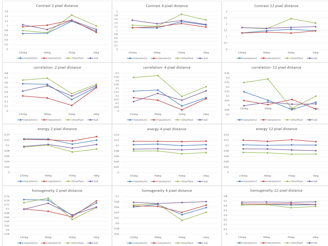
Figure 4. GLCM prosperities of 4 sample images in different angles and displacements.
