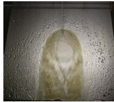
Fig. 1: Rust generated by flowing water. (45 min.)
