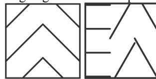
Figure 4: Assignment of patches to reflector pixels. Two and three patches are assigned in the left and right hand figures, respectively.
