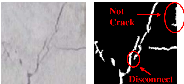
Fig2. A result of the detection method using wavelet transform [5]
