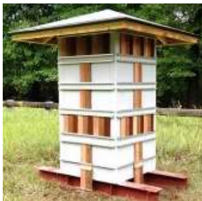
Figure 2. Exposure test stand frame
